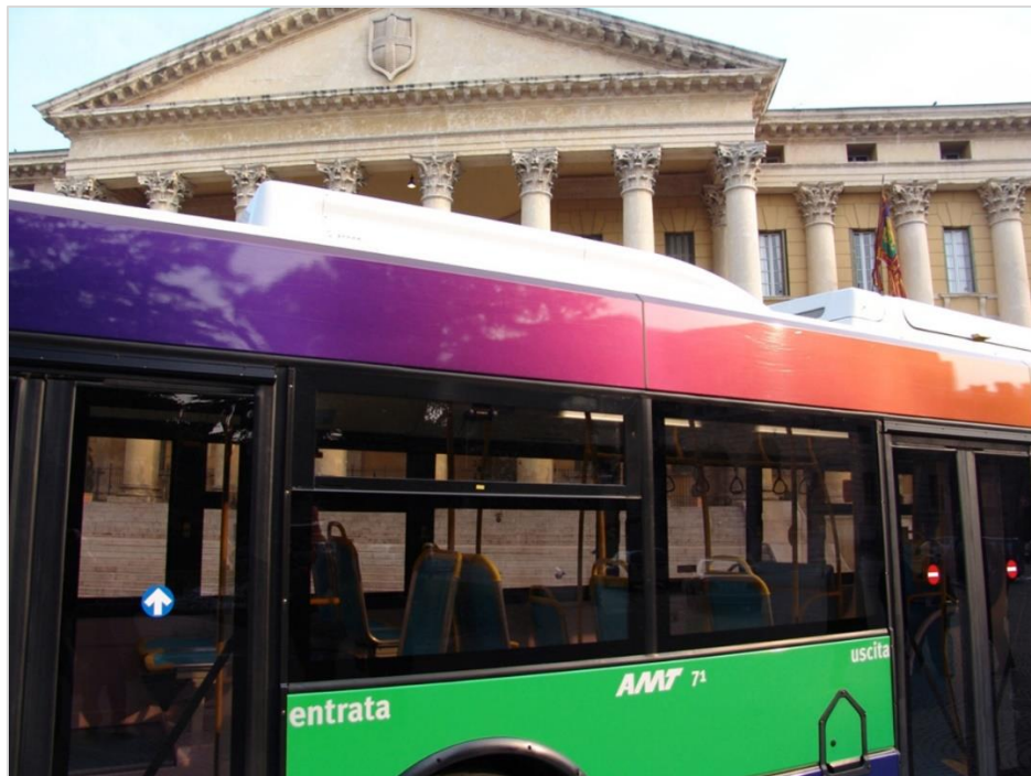
Fig 8: The vehicle body was divided in three in order to optimize the perception of the vehicle's dimension as well as to reduce its maintenance costs
